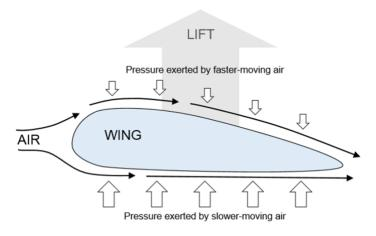
\*Optional: draw this wing diagram out to demonstrate the principle applied to aviation.
